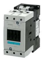
Contactor, AC-1, 140 A / 400 V, 230 V AC, 50 Hz, 3-pole, Size S3, Screw terminal !!! Phased-out product !!! Successor is SIRIUS 3RT2 Preferred successor type is >>3RT2446-1AP00<<
