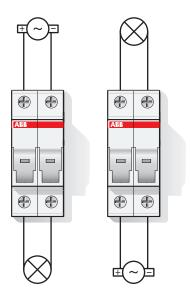
Wiring diagram for a.c. networks
