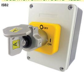
Power "ON" = Key TRAPPED. Power "OFF" = Key can be RELEASED
