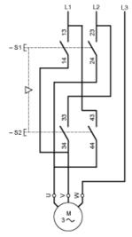
Combined with 3-pole isolating block XACS399 or XACS3991, shown in the unoperated position (pendant station "supplied"), fitted with key release trigger action
