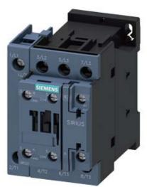
4NO CONTACTOR, AC1: 50A AC 110V 50HZ 4-POLE, 4NO, SZ: S0, SCREW TERMINAL 1NO+1NC INTEGR.
