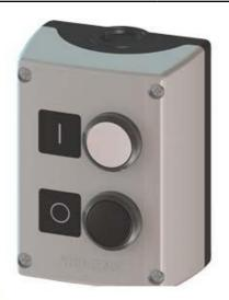
ENCLOSURE FOR 22MM PROGRAM PLASTIC VERSION 2 COMMAND POSITIONS GRAY TOP PART A=PUSHBUTTON BLACK,LABEL"O" 1NO B=PUSHBUTTON WHITE, LABEL "I" 1NC
