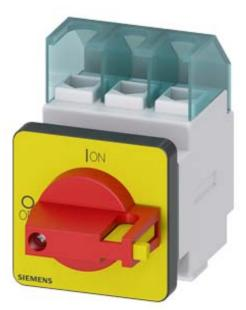
SENTRON, 3LD switch disconnector, EMERGENCY-STOP switch, 3-pole, lu:32 A, Operational power / at AC-23 A at 400 V: 11,5 kW, front- mounted, knob-operated mechanism, red/yellow, 4-hole mounting of the handle
