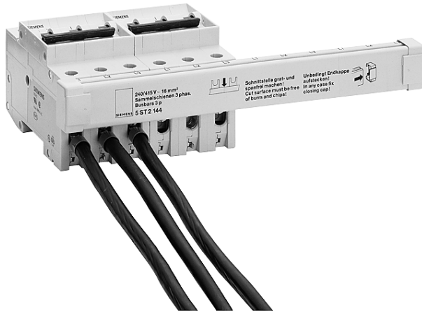
Simultaneous connection of the bottom feeder cables with cross-sections of up to 25 mm 2 and the 5ST2 144 3-pole busbar to the combined terminal of the miniature circuit-breaker.
