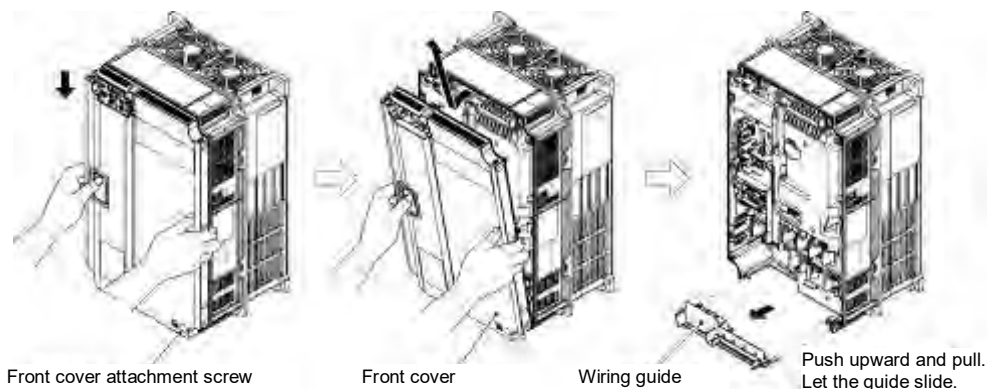
Figure 2.2-5 Removal of the Front Cover and the Wiring Guide (for VXT-72A-4)
