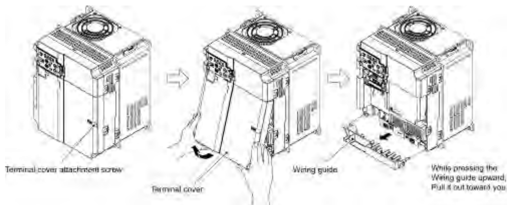
Figure 2.2-4 Removal of the Terminal Cover and the Wiring Guide (for VXT-69A-2)
