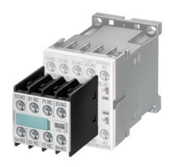
AUXILIARY SWITCH BLOCK, 22, 2NO+2NC, DIN EN50005, SCREW CONNECTION, F. CONTACTOR RELAYS A. CONTACT. FOR SWITCHING MOTORS, SIZE S00
