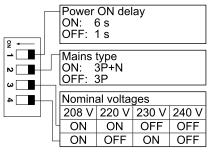
Fig. 1 DIP switch settings table M44
