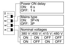
Fig. 3 DIP switch settings table M48
