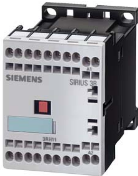
CONTACTOR RELAY, 3NO+1NC, AC 110 V, 50 HZ, CAGE CLAMP CONNECTION, SIZE S00
