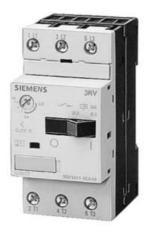
CIRCUIT-BREAKER SIZE S00, FOR MOTOR PROTECTION, CLASS 10, A-REL. 4.5...6.3A, N-REL. 82A SCREW TERMINAL, STANDARD SWITCHING CAPACITY
