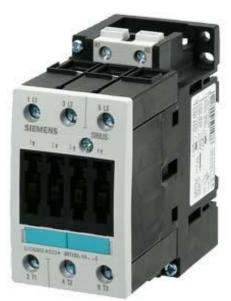
Power contactor, AC-3 40 A, 18.5 kW / 400 V 220 V AC, 50 Hz / 240 V, 60 Hz, 3-pole, Size S2, Screw terminal !!! Phased-out product !!! Successor is SIRIUS 3RT2 Preferred successor type is >>3RT2028-1AP60<<
