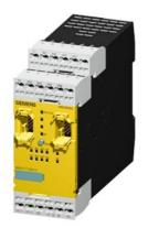
SIRIUS, central unit 3RK3 Basic for modular Safety system 3RK3 4/8 F-DI,1F-RO,1 F-DO,24 V DC parameterizable using software Safety ES 45 mm overall width Spring-type terminal Up to SIL3 (IEC 61508) Up to Performance Level E (ISO 13849-1)
