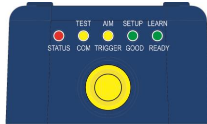
Figure 7 – X-PRESS™ Interface: Learn Function
