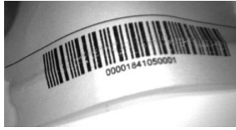
Figure 18 - Barcode Printed on Curved Surface Readable by Matrix 300N™ in spite of Image Optical Distortion
