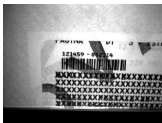
Figure 17 - Overprinted Barcode Readable by Matrix 300N™ also Through the Envelope Window Film
