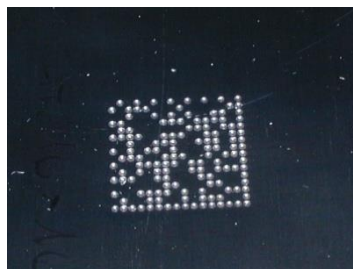
Figure 21 - Directly Marked Dot Matrix Code Characterized by Outstanding Separation Distance between Adjacent Code Elements
