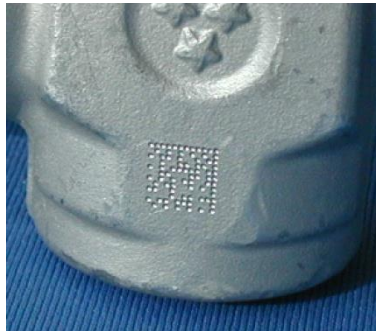
Figure 19 - Dot Matrix Code Directly Marked on Metal Surface by Using Dot Peening Technology
