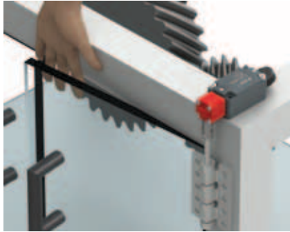
Verify the switching point according to EN ISO 13857 and recalibrate if necessary.
