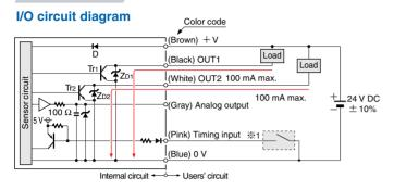
Note: If using together with an ionizer, the 0 V line of this product should be connected to the ionizer ground. In addition, the metal parts of the sensor head (EF-S1HS) are connected to the 0 V line, so it should be insulated during installation.
