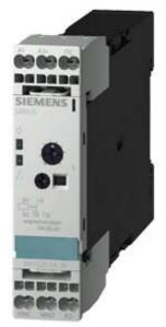
Timing relay, Multifunction Phased-out product !!! For further information, please contact our sales department Spring-type terminal 1 change-over contact, ansprechverzögert 0.05 s...100 h 24 V AC/DC/200...240 V AC at 50/60 Hz AC
