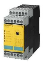
SIRIUS safety relay with relay enabling circuits (EC) 24 V DC, 45 mm overall width Screw terminal EC instantaneous: 2 NO EC delayed: 2NO, 0.05...3 s SC: 1NC AUTOSTART Basic device Maximum achieved SIL: 3/2, PL: e/d
