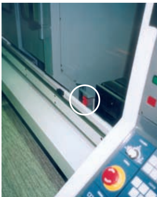
Example of use: TZK use on sliding doors of tool machines
