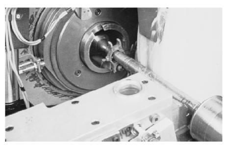
The Zero-Speed Controller monitors the rotation of the grinding wheel, and shuts the machine down immediately in case the drive shaft breaks.
