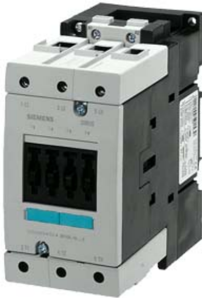
CONTACTOR, AC-3 37 KW/400 V, AC 230 V, 50 HZ, 3-POLE, SIZE S3, SCREW CONNECTION
